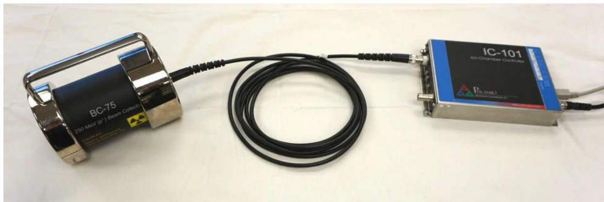
Figure 7. Connection to IC101 electrometer
